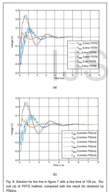
It is observed that if the rise time is increased, the shape of the pulses becomes smooth. Hence, the rise time is a very important factor to ensure that the signal will be stable as shown below:
