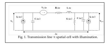
Consider a (n+1) conductor, uniform transmission line; the Telegrapher's equations of the MTL in the terms of total voltages, illuminated by an incident field are [1]:
